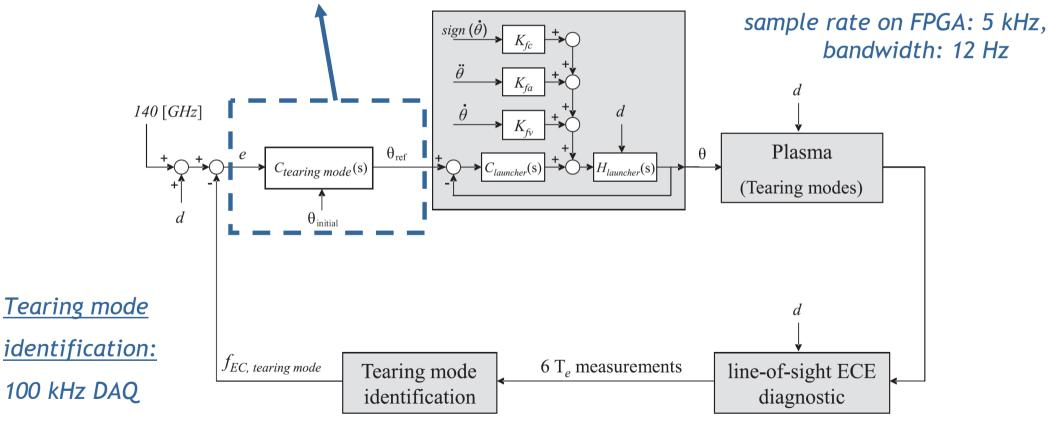
clock rate identification algorithm on FPGA: 16 μs
