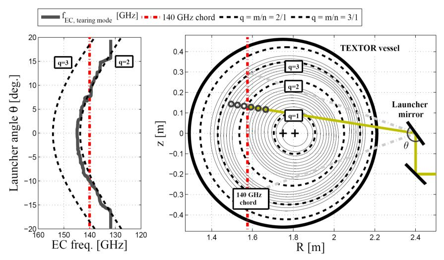
■ Match actuator frequency 140 GHz with sensor frequency  $f_{EC, tearing mode}$  GHz through launcher steering (elevation angle  $\theta$ )
