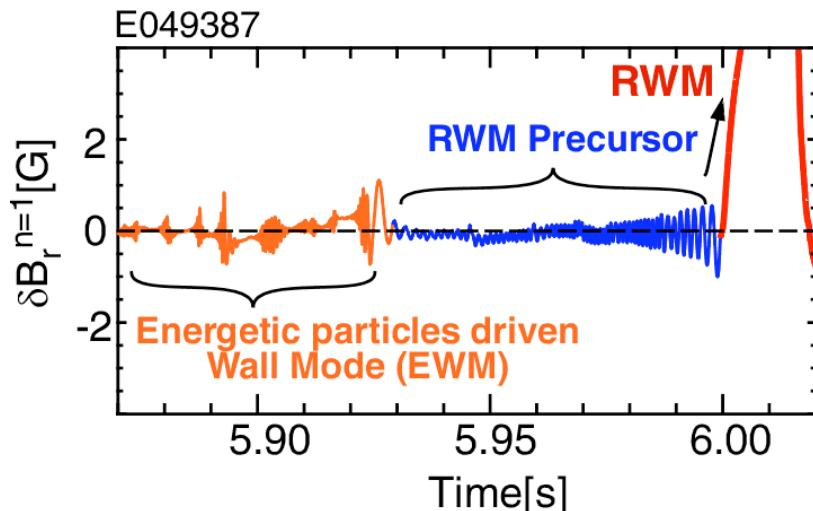
EWMs must be avoided to reduce risks to induce disruptions caused by RWM despite  $V_t > V_t^{\text{cri}}$ .
