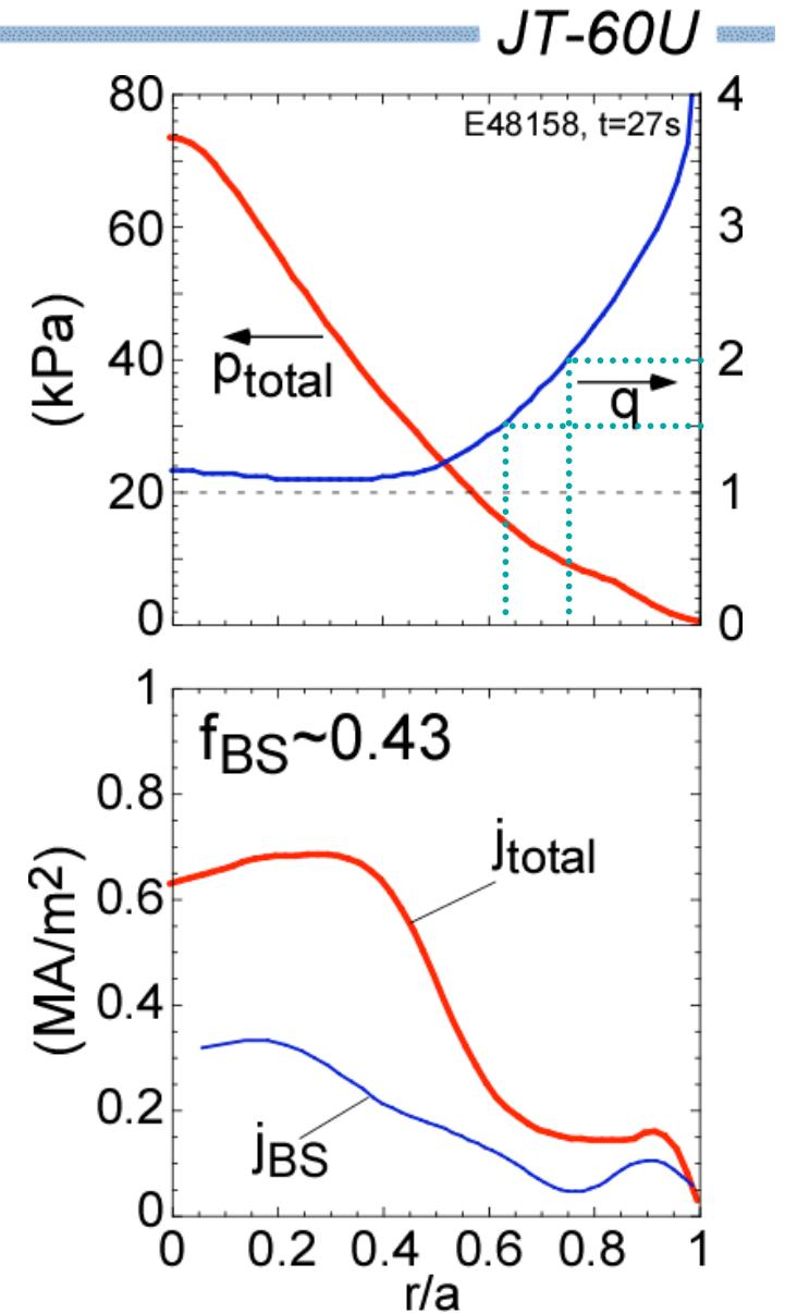
Peaked pressure has been kept with smaller  $P_{\text{net}}$  by central heating.  $\beta_N H_H > 2.6$  is sustained for 25s ( $\sim 14\tau_R$ ).
