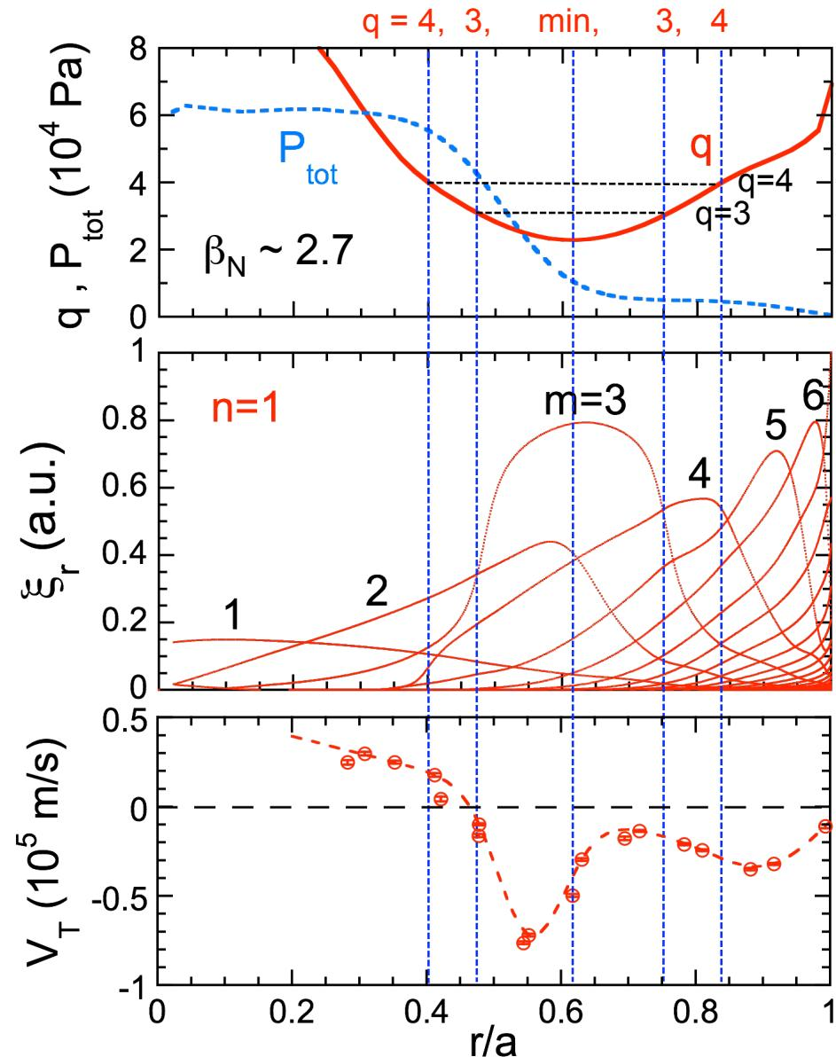
Toroidal rotation at the outer half of minor radius seemed to be important for RWM stabilization
