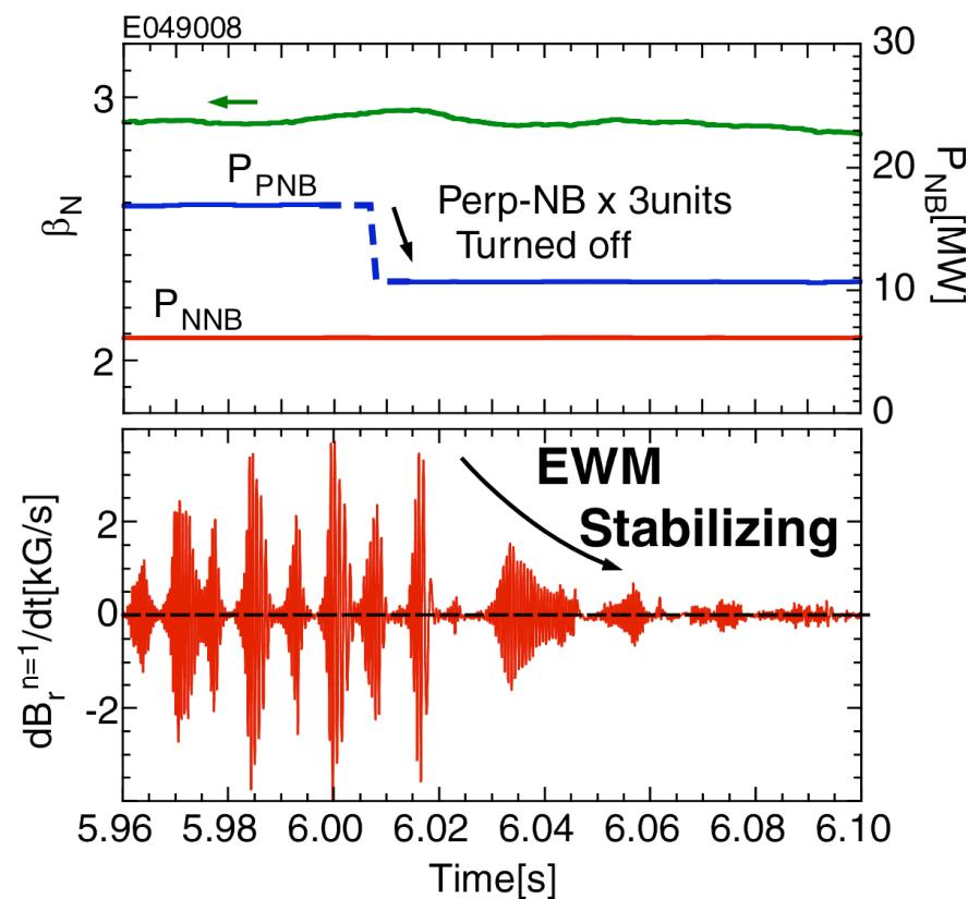
**EWM is destabilized by trapped energetic particle**
