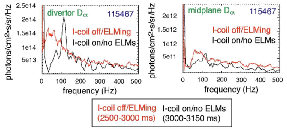
Type I ELMs at 30-100 Hz are strongly suppressed & the 130 HZ oscillatory envelope appears
