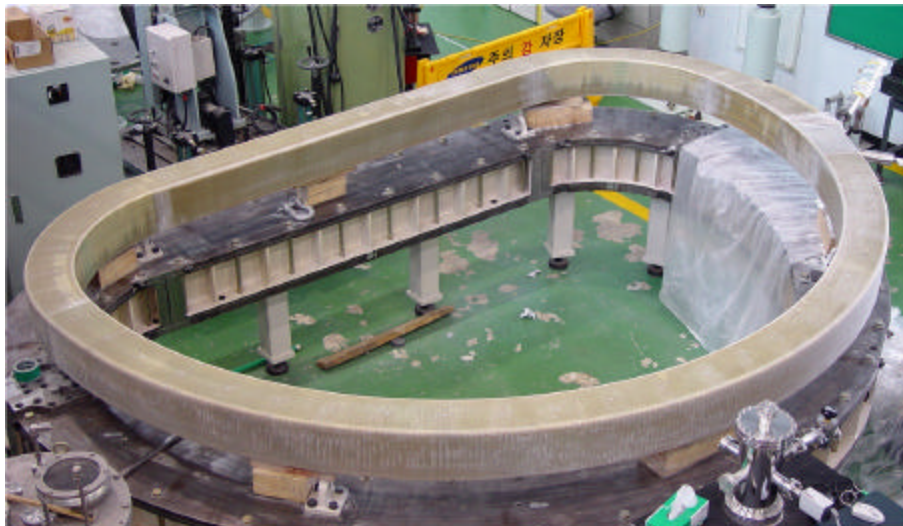
Fig. 6. Nb 3 Sn TF coil winding pack after winding, heat treatment, insulation and impregnation in the KSTAR Magnet Fabrication and Test facility
