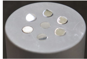
Divertor Material Evaluation System (DiMES)
