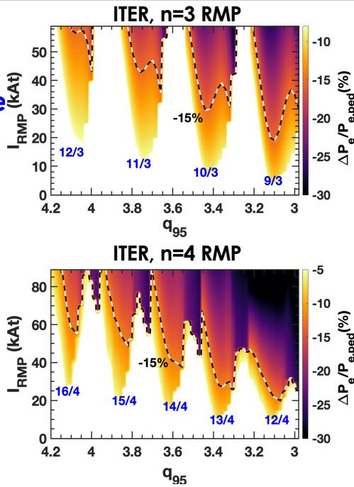
**Prediction and optimization of threshold field and  $I_p$  range for ELM suppression in ITER**
