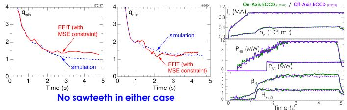
Increases confidence in steady-state Q ≥ 5 ITER hybrid scenario using off-axis current drive
