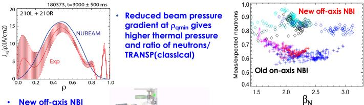
New off-axis NBI current drive matches simulations
