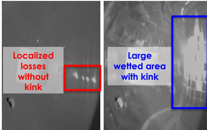
Path to RE energy dissipation over large area on resistive timescale, without CQ regeneration
