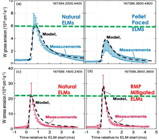
Intra-ELM W gross erosion reduced with pellet pacing but increased with RMP
