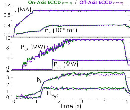
Increases confidence in steady-state  $Q \geq 5$  ITER hybrid scenario using off-axis current drive
