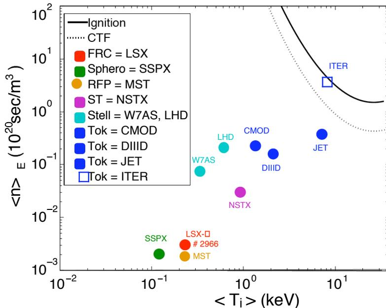
Fig. 2-6. Achievements of the various concepts relative to the goal of reaching fusion conditions.
