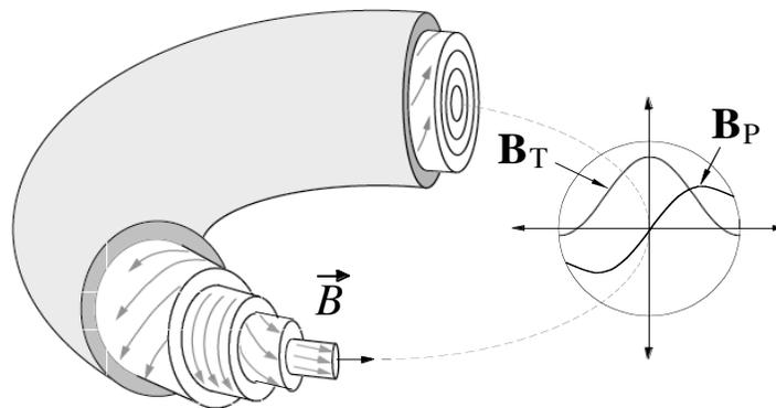
Fig. 6-1. The RFP magnetic configuration. The poloidal field inside the plasma,  $B_p$ , is comparable to the toroidal field,  $B_T$ , which is reversed compared to the small external toroidal field provided by the TF magnets.
