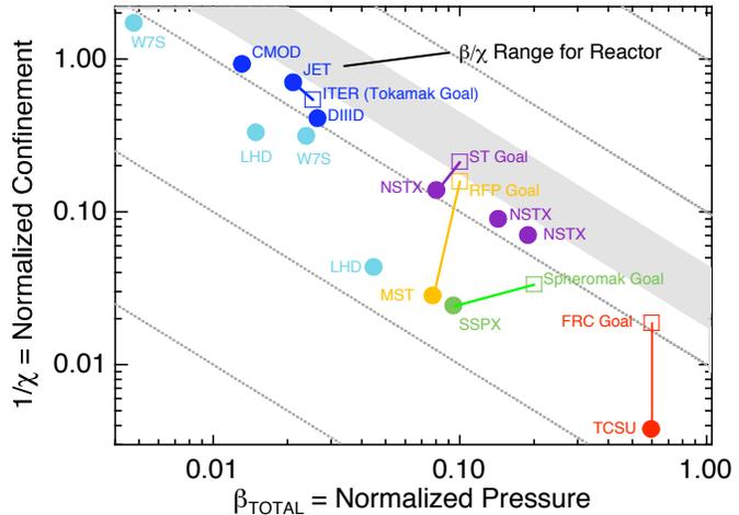
Fig. 2-7. Normalized performance of the various concepts in terms of  $\beta/\chi$  as above.
