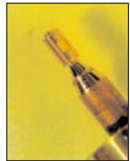
Final Machined Plastic-coated Gold Hohlraum on Copper Mandrel
