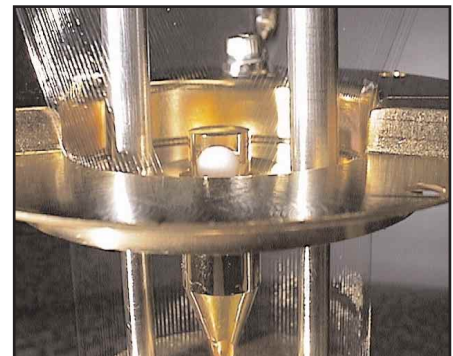
Fig. 2: A 12 degree vertical view of the “Javelin” target installed within the wire array. This view is similar to that of diagnostic instruments.
