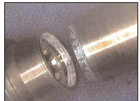
Test of a 9° taper seal with indium gasket, showing indium well bonded to both seal surfaces
