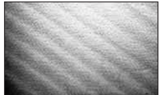
Fig. 2: Plastic film with \sin(x) perturbation (0.25 \mu\text{m} amplitude and 12.5 \mu\text{m} period)
