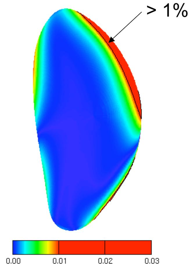
At finite  $\beta$ 's ripple contours permeate somewhat further into core (i.e., ripple amplification by diamagnetic currents)
